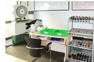
▲ 扭转试验机 [10000N.m] (行业首台) ▲ Torsion testing machine [10000N.m] (First in the industry)
